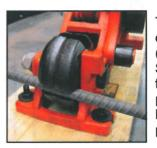
The bottom cutting slot is designed for cutting both #4 (1/2") and #3 (3/8") rebar. Simply put handle in the forward upward position and place rebar for desired cut. Make sure the rebar is fully placed into the cutting slots.
