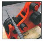
The top cutting slot is designed for cutting both #5 (5/8") and #4 (1/2") rebar. Simply put handle in the forward upward position and place rebar for desired cut.
